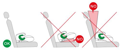
Check whether the safety seat is installed correctly. Proper installation is crucial to ensure the safety of children. The fixing of the child seat must follow the instructions on the belting stickers located on both sides of the seat or the instructions in the manual.
