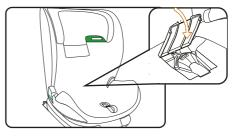
Place the shoulder strap behind the headrest cover, open the cover of buckle storage, assemble the buckle properly, then put it in the storage and close it.
