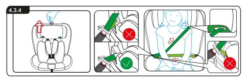
Adjust the height of the headrest to suit your child. Put the vehicle belt through the belt guide. Place your child into the baby car seat and let the vehicle belt pass the belt guide. Fasten the vehicle belt with an audible "click" sound.
