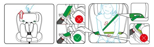
Adjust the height of the headrest to suit your child. Put the vehicle belt through the belt guide. Place your child into the baby car seat and let the vehicle belt pass the belt guide. Fasten the vehicle belt with an audible "click" sound.
