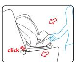
Grasp the seat body to check the seat if it is fastened tightly or shakes, meanwhile observe the ISOFIX red/green indicator. If the seat shakes and the ISOFIX connectors are pulled out, please repeat the above steps and install it again.
