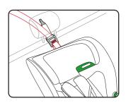
Hook the tether strap hook onto the user-ready anchorages. There may be 3 anchorages for the hook, please find one most suitable.
