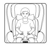
Please note a correctly adjusted headrest ensures optimal protection for your child in the safety seat; the headrest must be adjusted so that the shoulder straps are at the same level as your child's shoulders or slightly above.
