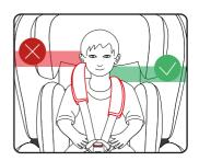
Guide the two buckle latches together and engage them before putting them into the buckle, this should make a clicking sound.
