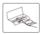
Pull the tether strap on the other end back to tighten the top tether.
